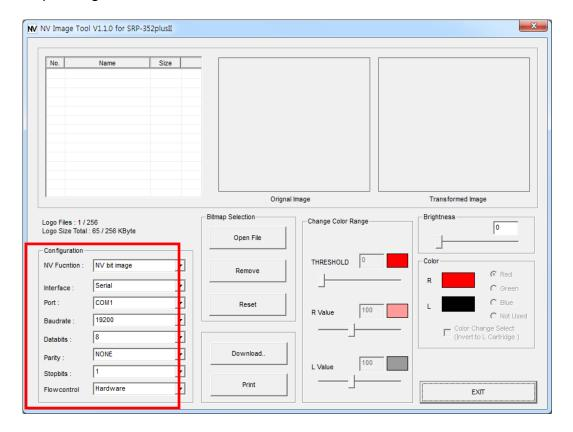
\* In the Serial Interface, match the communication setting (COM port number and Baudrate) to those of the printer.
